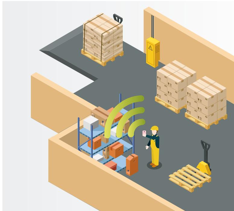
Beacons also operate as temporary devices. The installation is flexible and easy. Colored Beacons are used to provide better visibility. The innovative battery technology provides two to eight years of service without reverting from external energy sources.
