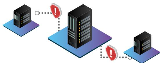
The Node can be started in field environments and act as a standalone Fallback mode server. Furthermore, the node can be configured as a part of the TASSTA cluster and be connected to the system back on link availability.
