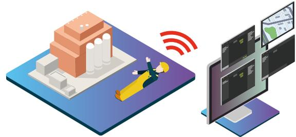
An effective way to make a pathway of workers safer. Being active, the app uses GPS location data obtained from a mobile device to detect a user movement. If a user remains motionless for a certain period of time, an Inactivity Timer will start. If there is still no movement, the application sends an Emergency Alert and automatically initiates an Emergency Call.
